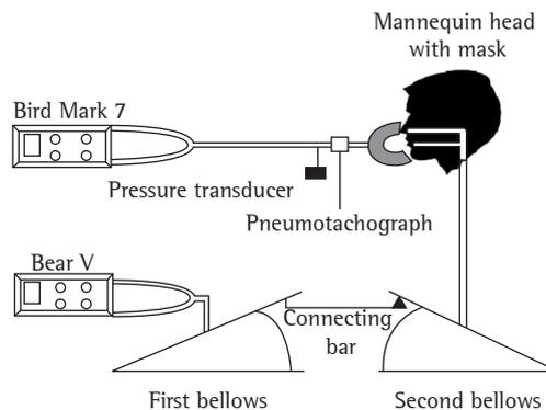
**Figure 1** - Illustration of the experimental model with the Bird Mark 7 and the Bear V (mechanical ventilator used to simulate the inspiratory pressure). The first and second bellows constitute the simulator of the respiratory system.
