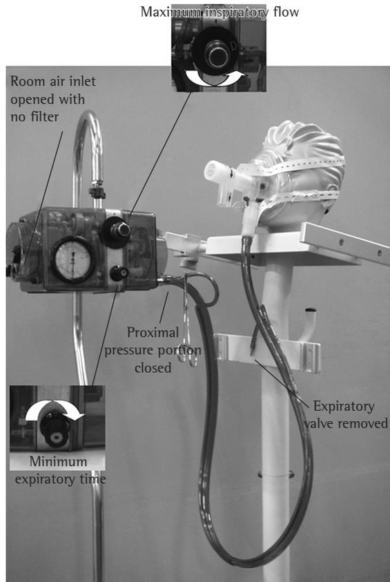
**Figure 2** – Bird Mark 7 adapted to offer continuous positive airway pressure. The expiratory time (lower) dial was turned clockwise as far as possible. The inspiratory flow (upper) dial was turned counter-clockwise as far as possible. As can be seen, the proximal pressure portion of the circuit was clamped with surgical forceps.
