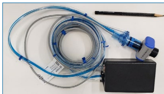
Figure 2. Photograph of our portable volumetric capnograph with sensors and connections.
